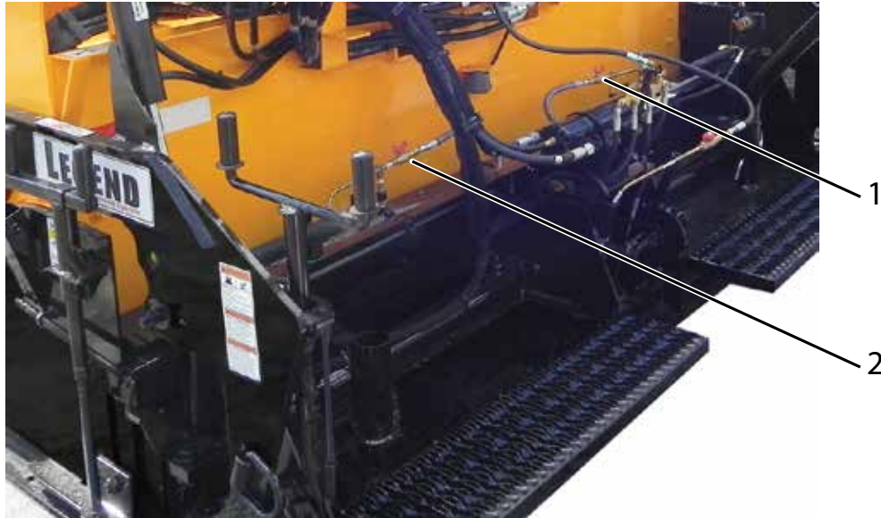
Figure 3-8. Extension Burner Controls
