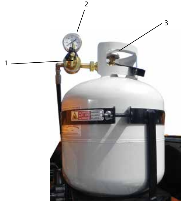
Figure 4-4. Propane Tank With Regulator
