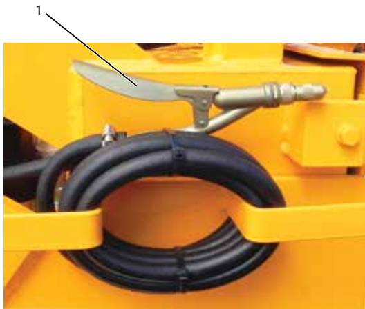
Figure 4-3. Spray Down Hose
