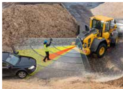
Reversing camera with radar detect
