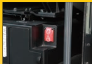
Emergency engine stop switch
