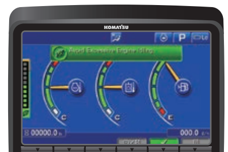
Eco-gauge, Eco guidance and fuel consumption gauge
