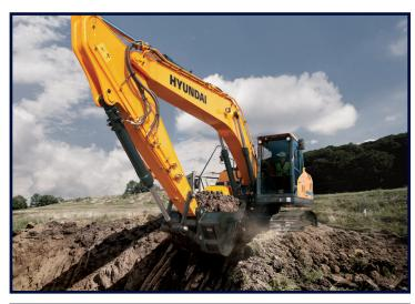
Operating weight, including 5,680 mm (18' 8") boom, 2,920 mm (9' 7") arm, SAE heaped 0.92 m³ (1.20 yd³) bucket, lubricant, coolant, full fuel tank, full hydraulic tank, max 4,500 kg (9,920 lb) counterweight and all other standard equipment.
