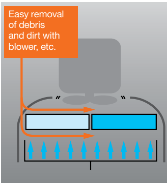
Parallel arrangement of radiator and oil cooler
