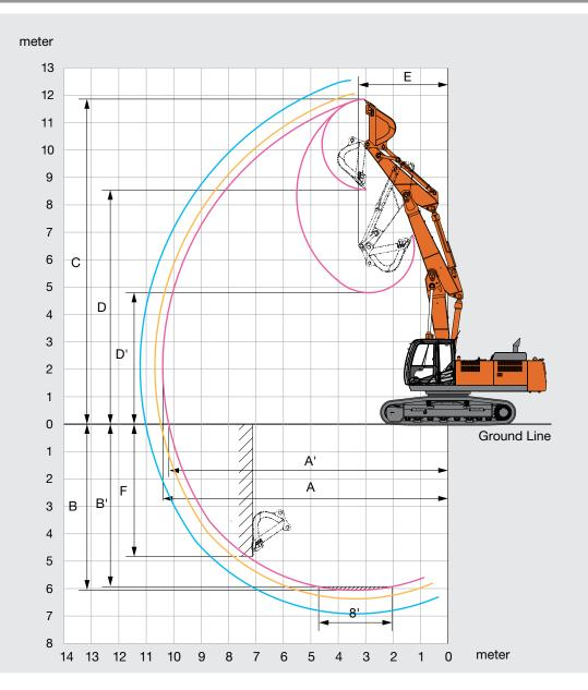
ZAXIS 350LC / ZAXIS 350LCN 6.39 m 2-Piece boom 3.20 m 2.33 m 2.67 m Arm length 10 390 10 680 11 220 A Max. digging reach 10 170 10 470 11 020 A' Max. digging reach (on ground) B Max. digging depth 6 040 6 360 6 900 B' Max. digging depth (8' level) 5 930 6 800 6 250 C Max. cutting height 11 870 12 060 12 550 D Max. dumping height 8 550 8 750 9 2 4 0 D' Min. dumping height 4 810 4 330 3 650 E Min. swing radius 3 250 3 120 2 890 4 820 5 090 5 780 F Max. vertical wall digging depth
