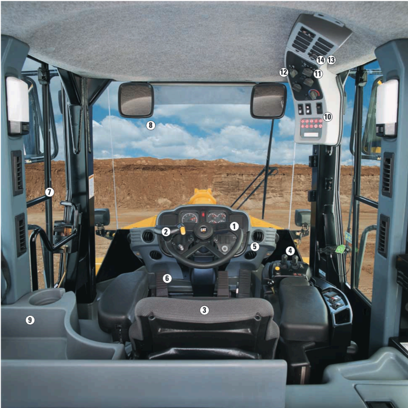
Command Control Steering with Electro-Hydraulic Bucket Controls
