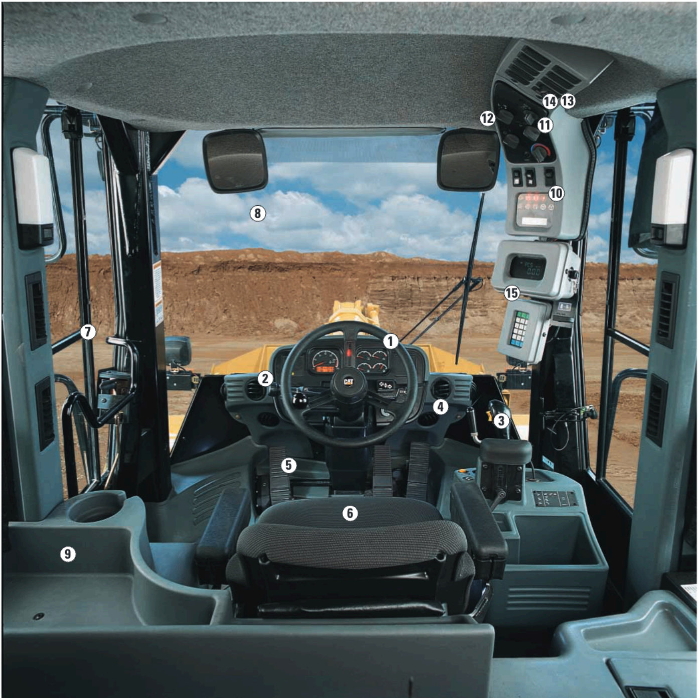
Conventional Steering Wheel (SW) with Pilot Hydraulic Bucket Controls
