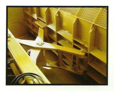
E series scrapers are the largest ejector finishing scrapers manufactured. All E scrapers are equipped with our signature scissor ejection system. The wheel frame with 20.5 x 25 tires provides superior flotation and clearance while leveling.
