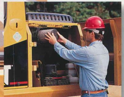
A standard Cat Radial Seal Air Filter requires no tools – for fast removal or installation.
