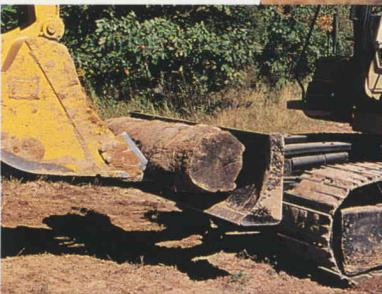
New optional blade makes the machine perfect for carrying, clearing, backfilling, and grading.
