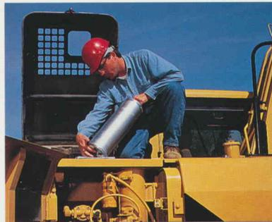
Hydraulic oil cartridge filter is located outside the hydraulic tank, making filter changes fast and clean.
