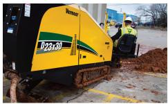
COMPACT YET POWERFUL. The D23x30 S3 features a short, narrow design, while its 100 hp (75 kW) Deutz engine offers the power operators need when working in tough ground conditions.
