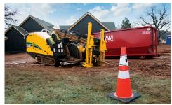
MAXIMIZE PRODUCTIVITY. With 24,000 lb (106.8 kN) of thrust/pullback and 3000 ft-lb (4067.5 Nm) of rotational torque, the D23x30 S3 offers a sizeable increase in power over its predecessor, the D20x22 Series II — helping to maximize machine and jobsite productivity.
