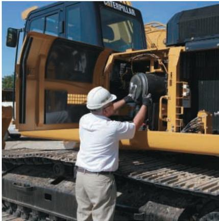
**Air Filter Compartment.** The air filter features a double-element construction for superior cleaning efficiency. When the air cleaner plugs, a warning is displayed on the monitor screen inside the cab.
