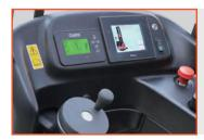
•Multi-function color LCD instrument can display information such as steering wheel position, battery power, power alarm, fault code, running time, driving speed etc.
