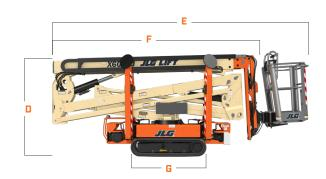
A. Platform Width 30-in / 76-cm B. Platform Length 58-in / 1.47-m Machine Width\* 31-in / 78-cm ۵. Machine Height 6-ft 6-in / 1.98-m E. Machine Length 16-ft 5-in / 5.01-m F. Machine Length Without Platform 15-ft 3-in / 4.65-m G. Track length 4-ft 10-in / 1.47-m H. Outrigger Footprint - Length 10-ft 7-in / 3.22-m I. Outrigger Footprint - Width 10-ft 7-in / 3.23-m J. Outrigger Pad Diameter 11.8-in / 30-cm
