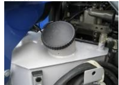
Filler on fuel tank in superstructure
