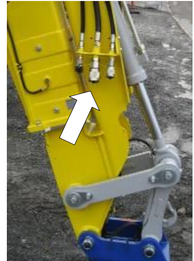
Connection at boom on the right side
