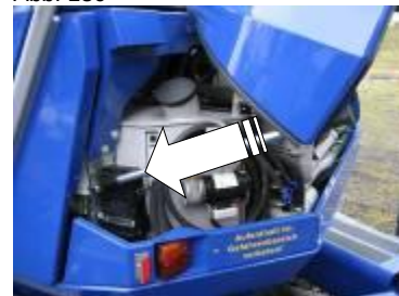
Insert the pump lever
