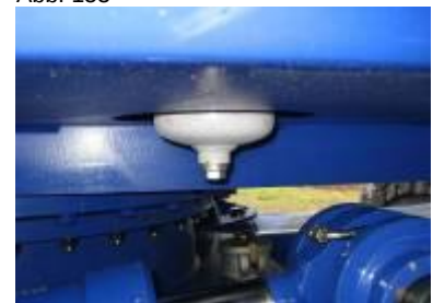
Drain bolt fuel tank
