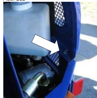
Rear fastening of the radiator cover
