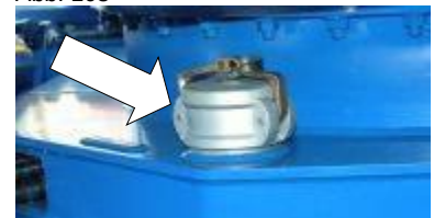
Filler of spare diesel tank
