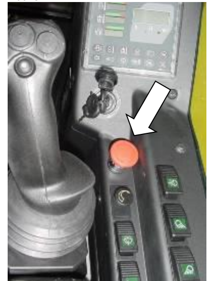
Location of emergency pushbutton in the cab
