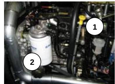
Engine oil filler cap
