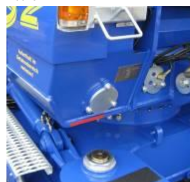
Location of nameplate or, respectively, CE label
