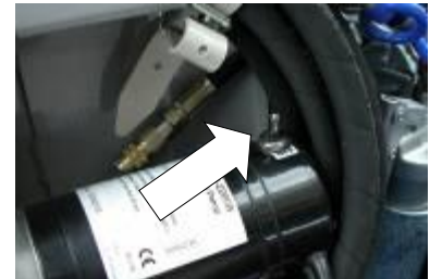
Switch of fuel pump
