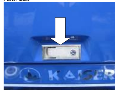
Closing the engine hood
