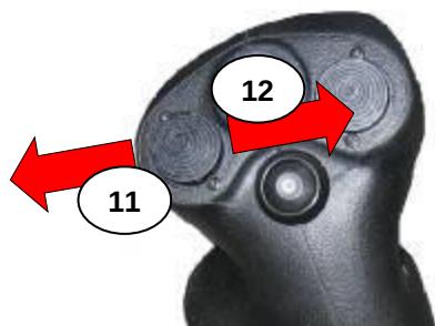
Abb. 83 Right pad leg / wheel OUT-IN (basic drawing)
