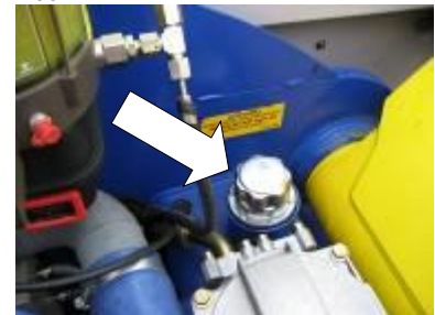
Hydraulic oil filler cap
