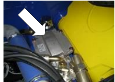
Hydraulic oil filter
