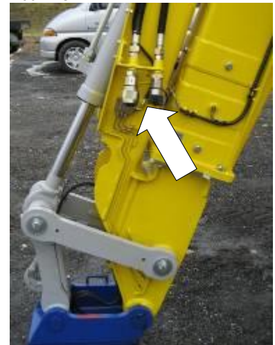
Connection at boom on the left side - General view
