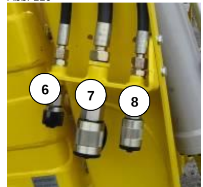
Connection at boom on the right side
