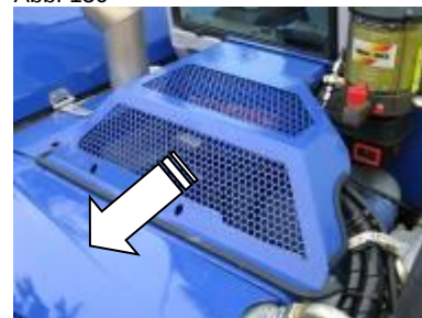
Removing the coarse filter
