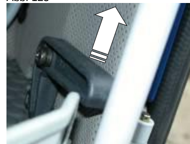
Door release lever in the cab
