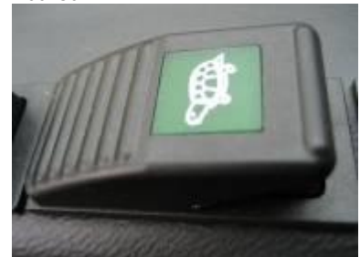
Switch for slewing, slow speed
