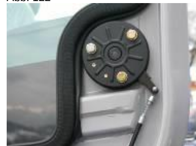
Door locking on the outside of the cab
