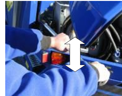
Operating the pump lever
