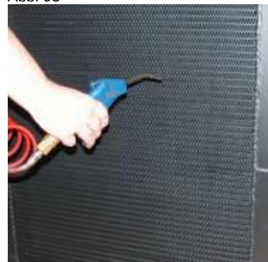
Cleaning the radiator by means of compressed air
