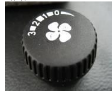
Blower speed switch
