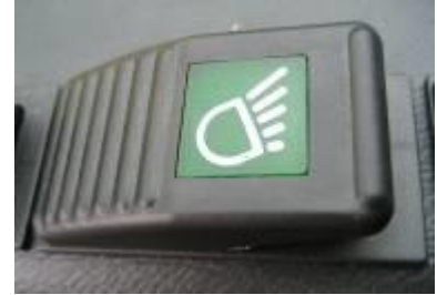
Rear working flood light
