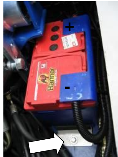
Position of battery 1
