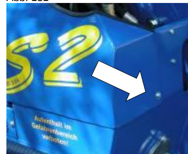
Front fastening of the radiator cover
