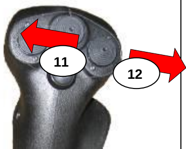
Abb. 76 Left pad leg / wheel OUT-IN (basic drawing)
