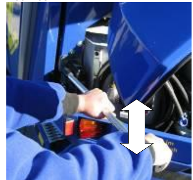
Operating the pump lever
