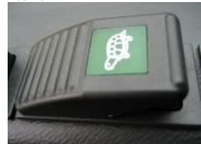
Switch for driving, slow speed
