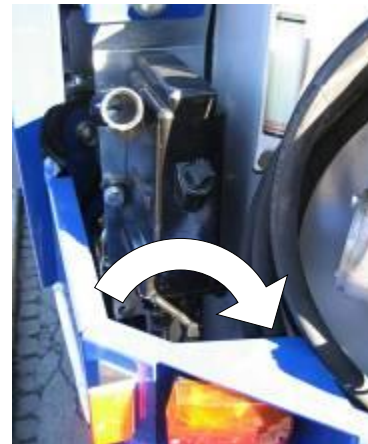
Set manual pump to LIFT
