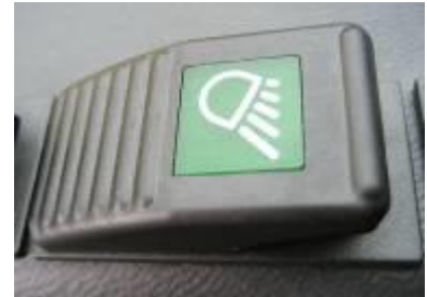
Working light, boom
