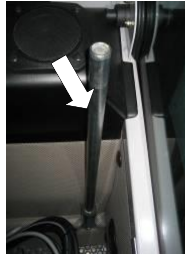
Storage place of the pump lever for the cab tilt pump
