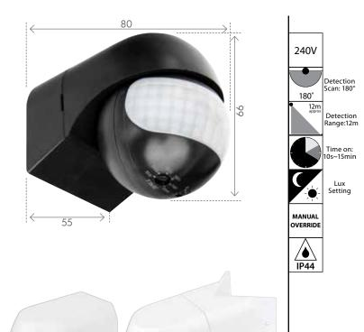
Passive Infra-red technology. Multi-segmented lens for better detection. Adjustable sensing angle. Reliable 3-wire design. Adjustable time and lux level. Manual override. IP44 weather-resistant rated. Resets to AUTO mode after 8 hours Wall mount Lux control level : 3-2000LUX (adjustable) Max Load : 800W Incandescent Lamp 400W Fluorescent Lamp 200W LED Lamp 2 Year Warranty.
