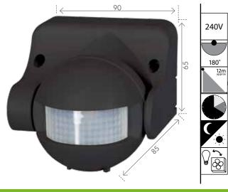
Passive Infra-red technology Multi-segemented lens for better detection 3-Wire design for greater reliability IP44 Weatherproof Rated Max Load: 300W Incandescent 100W Inductive Operating Temp: -5 to 45 degrees Celsius 2-Year Warranty
