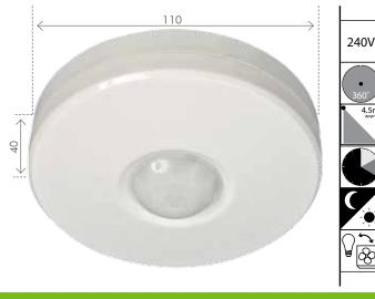
Passive Infra-red technology Surface mount for interior or exterior use Multi-segemented lens for better detection 3-Wire design for greater reliability IP44 Weatherproof Rated Max Load: 1600W Incandescent 500W Fluorescent 300W Inductive Operating Temp: -5 to 45 degrees Celsius 2-Year Warranty
