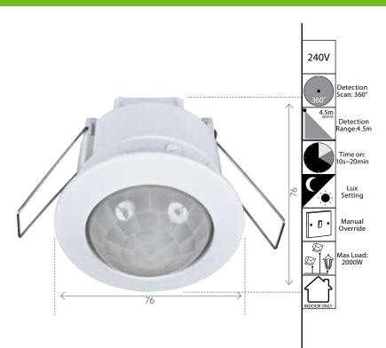
Passive Infra-red technology Recessed/Flush mounting Multi-segmented lens for better detection 3-Wire design for greater reliability Automatic Reset Time: 8 hours Max Load: 2000W Incandescent 600W Fluorescent 300W LED
