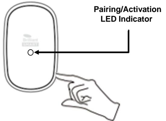
2. Press the Bell Press once, the LED indicator light on the Chime/Receiver will go Off, and the pairing will be complete
