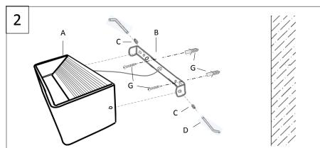
Remove mounting bracket 'B' from fitting body 'A' by undoing grub screws 'C' from both sides of the fitting with Allen key 'D' provided. Drill two holes in the wall using the holes in the mounting bracket 'B' as a template. Use screws and suitable fixture system 'G' to install the bracket onto the wall securely.
