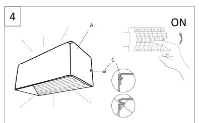
Fit fitting body 'A' onto mounting bracket 'B' installed on the wall with 2 x grub screws 'C' removed earlier. Gently tighten the grub screws up to the level with body 'A'. NOTE: Do not drive the grub screws too far inside the base beyond the surface of the body.
