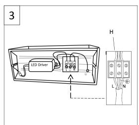
Feed mains supply cable through the wall and connect supply cable to terminal block 'H' according to the marking on it:
