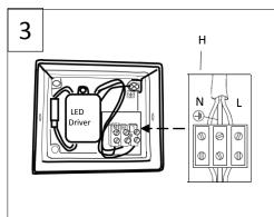
Connect supply cable to terminal block  $\,{}'\!H'$  according to the marking on it :
