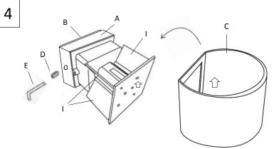
Fit fitting body 'A' onto mounting base 'B' and secure it on with 2 x grub screws 'D' removed earlier with Allen key 'E' provided. Adjust 4 x flaps 'I' to desired position. Slide decorative cover 'C' onto the fitting 'A' from the TOP. Refer to the 'UP arrow on it for correct orientation. Ensure it fits securely.
