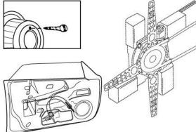
Mounting of the grommet on the inside panel.
