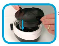
2. Place the Intake Cover Plug - seating it on the bottom flange and aligned to the left of the notch on the blower (verify that the intake plug gasket is free of debris).
