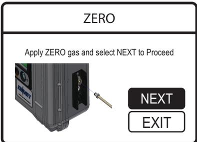
Connect the regulator to the calibration port on the side of the AirGuard.
