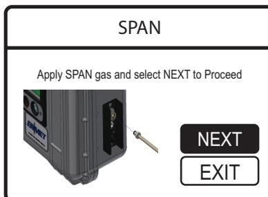
Upon selecting the "NEXT", AirGuard will display a "Span in Progress" display with a timer which counts down the time remaining in the span function.
