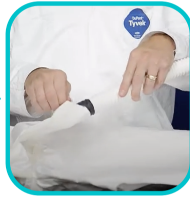
Insert breathing tube 12cm into the hood
