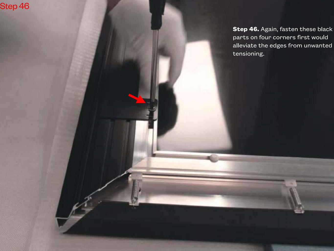
**Step 47.** Again, fasten these black parts on four corners first would alleviate the edges from unwanted tensioning.
