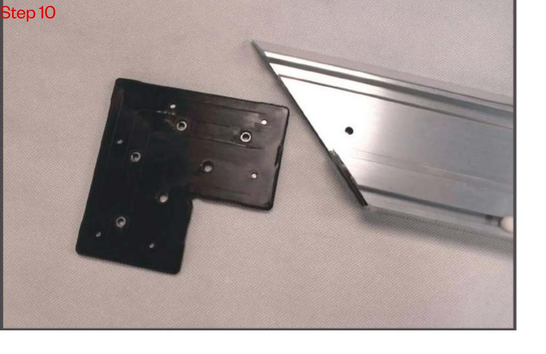
**Steps 10-12.** Assembly of corner connection parts: place corner parts inside the silver frame and connect the counter part, make sure the holes are aligned properly. When installing the two corner pieces, this should be done simultaneously and inserted at the same time. See images for reference
