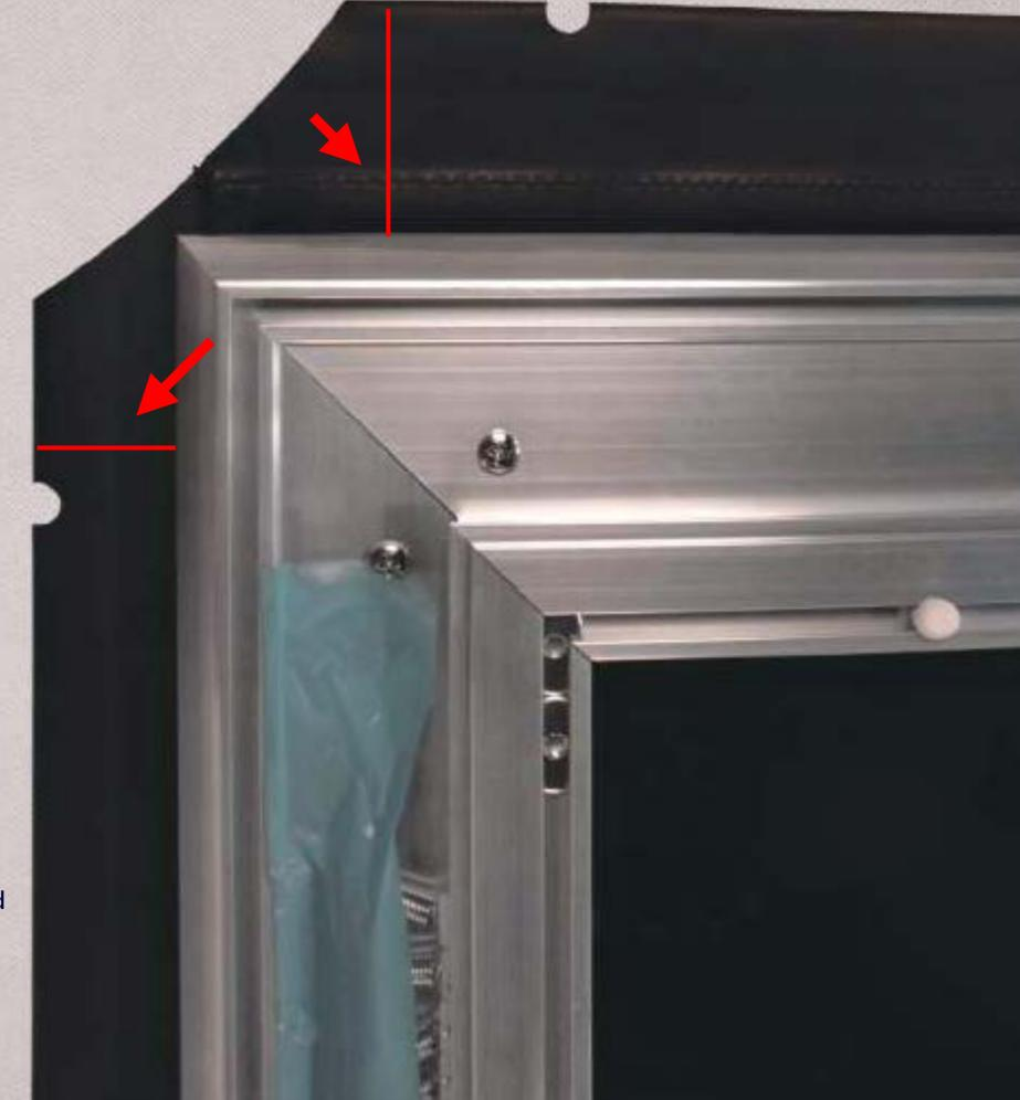
**Step 28.** This is to show you what a WRONG installation would look like, clearly both sides are not aligned properly, the silver frame here is not aligned with the dotted line.
