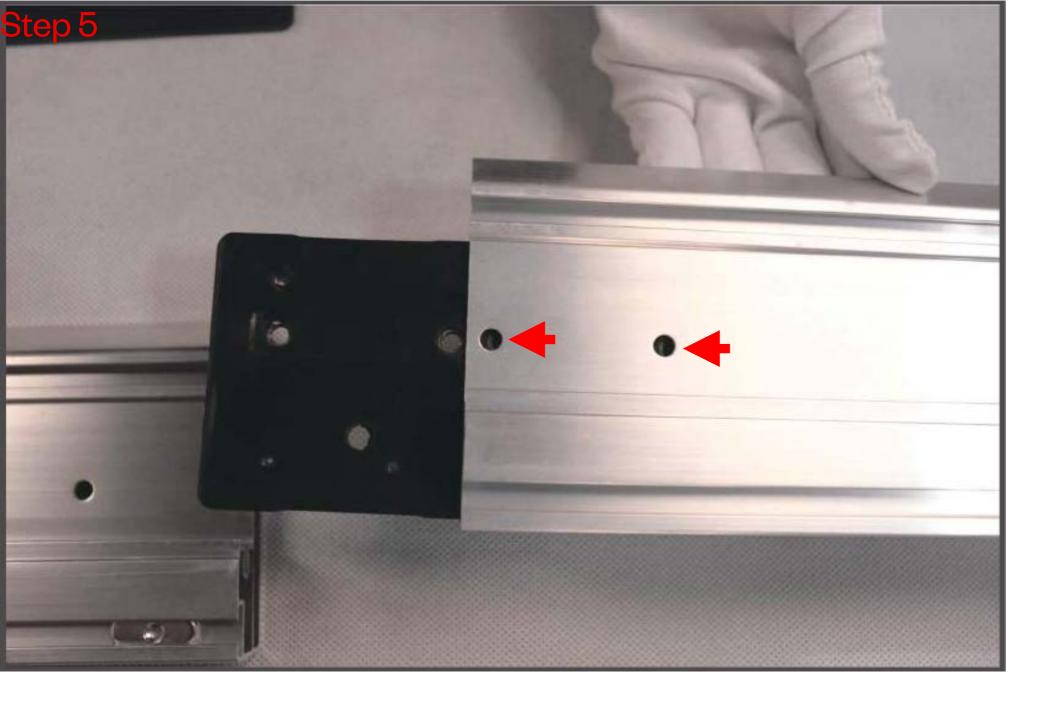
**Steps 5-8.** Align with the holes on both sides and securely fasten with screw. See images for reference
