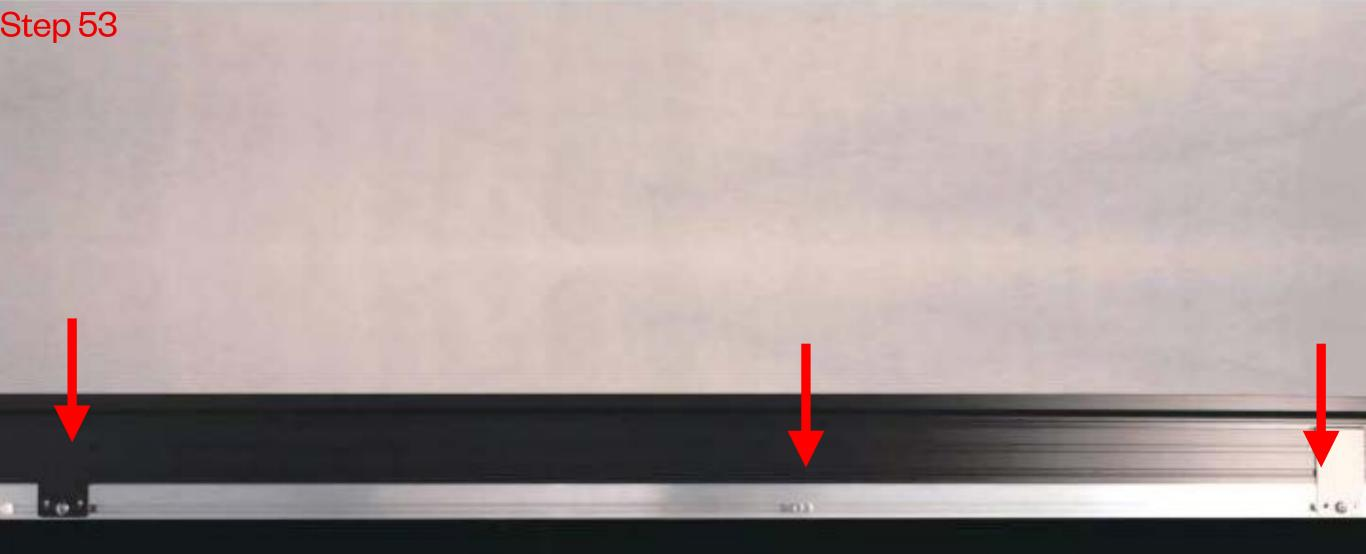
**Step 53.** Please leave the middle nut out of the three on there and the remainder nuts can be screwed with the black fastening pieces.
