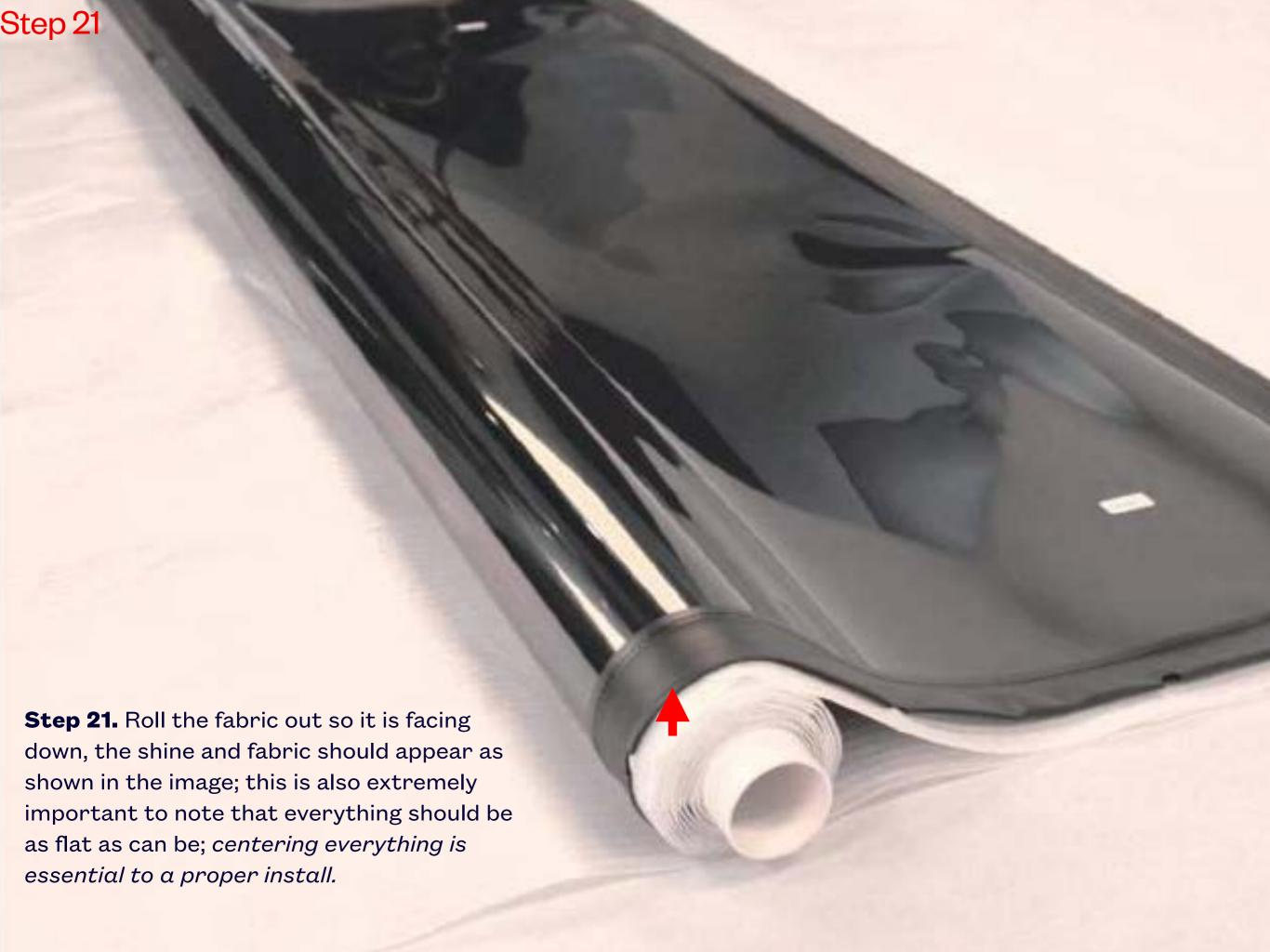
**Step 22.** As you roll out the fabric and make sure you pull the fabric at the same time from left and right. *Again, it is crucial that this is flattened out as much as possible and centered as you begin to unroll the fabric.*
