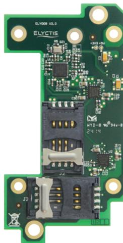
As an option, a secondary board offers an extension of two additional SAM slots.
