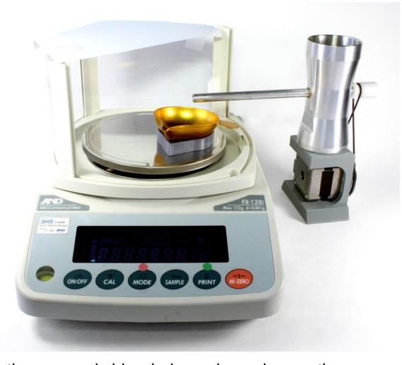
It is recommended to use the rear and side wind panels, and cover the top with a sheet of paper.
