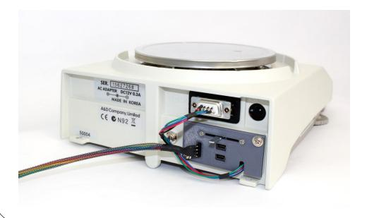
Insert the electronics and attach the connectors as shown.
