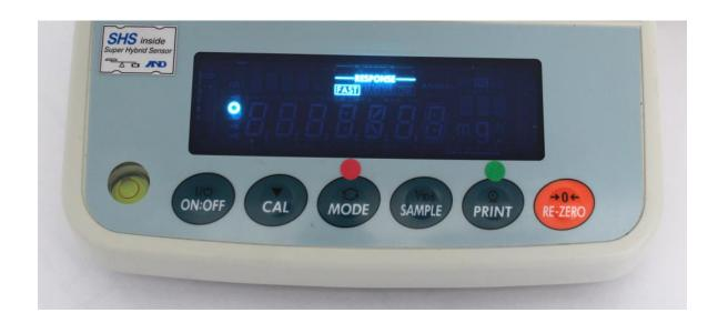
Set primary unit to grains (GN) and secondary unit to grams (g)
