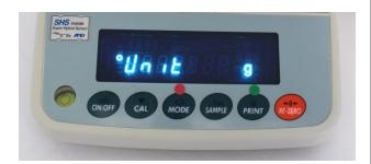
To check, turn the scale off and on and the unit should be **GN**. Then press MODE repeatedly and it should switch between **GN** and **g**.
