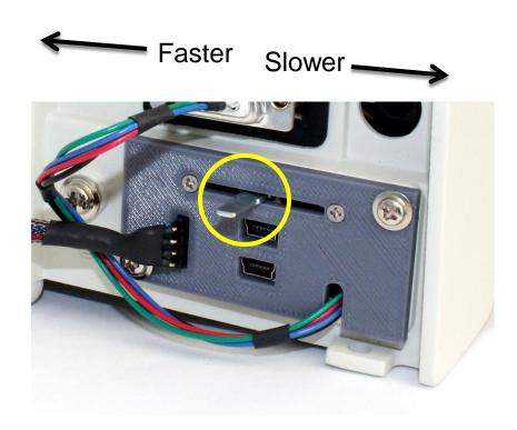
The trickler will be more consistent if the slider is near the middle. Adjust the tilt of the mount first, and use the slider for fine tuning.
