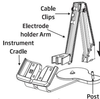
Slide edge<sup>DO</sup>® into the cradle while positioning the probe cable behind the cradle. Put the probe/sensor into the electrode holder and secure cable in clips.
