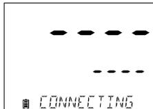
Connect the 3 mm probe jack to the probe input located on the bottom of edge<sup>DO</sup>®. **Make sure the probe is completely connected.** If the probe is recognized, "CONNECTING" message is displayed along with sensor model.
