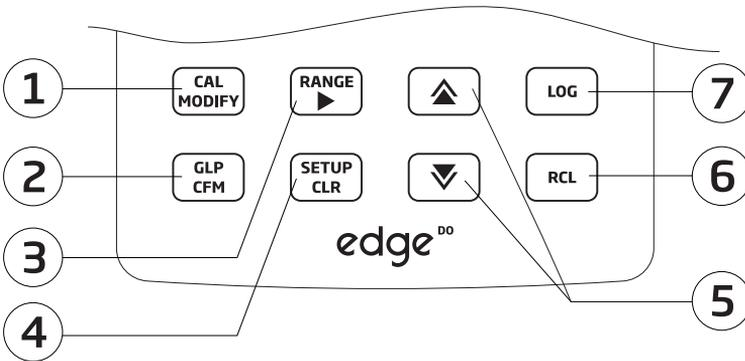
**1. CAL/MODIFY** - Used to enter and exit **calibration** mode. In SETUP, used to initiate changes of a configuration setting.
