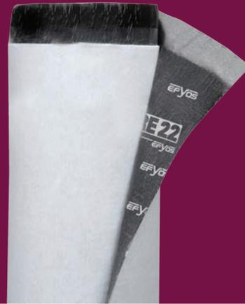
**VELAPHONE is an acoustic membrane made of polyester felt and a vapour barrier film (black film). It is specially designed to be mainly used on wood structures under a layer of 1½ in (38 mm)-thick self-levelling concrete.**
