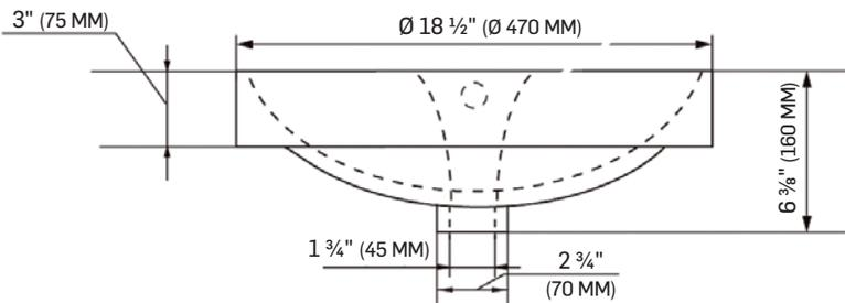
\* TOUTES CES DIMENSIONS SONT APPROXIMATIVES. AFIN D'ASSURER UNE INSTALLATION PARFAITE, LES DIMENSIONS DE LA STRUCTURE DOIVENT ÊTRE VÉRIFIÉES À PARTIR DE L'UNITÉ AVANT L'INSTALLATION.
