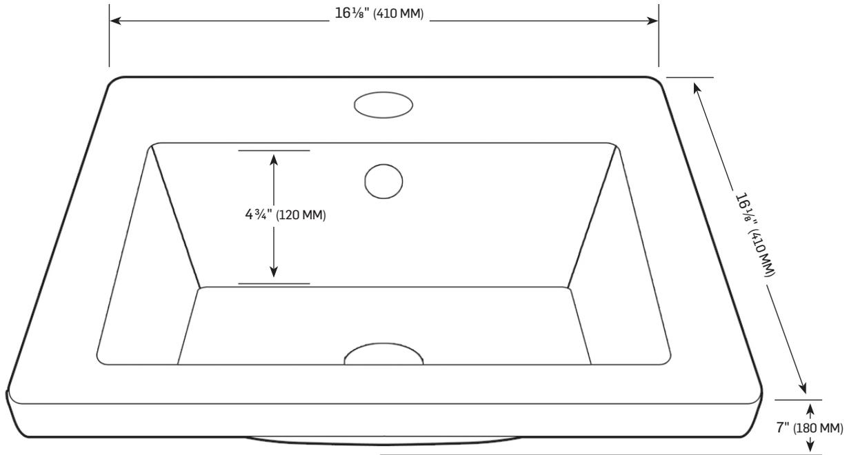
\* TOUTES CES DIMENSIONS SONT APPROXIMATIVES. AFIN D'ASSURER UNE INSTALLATION PARFAITE, LES DIMENSIONS DE LA STRUCTURE DOIVENT ÊTRE VÉRIFIÉES À PARTIR DE L'UNITÉ AVANT L'INSTALLATION.
