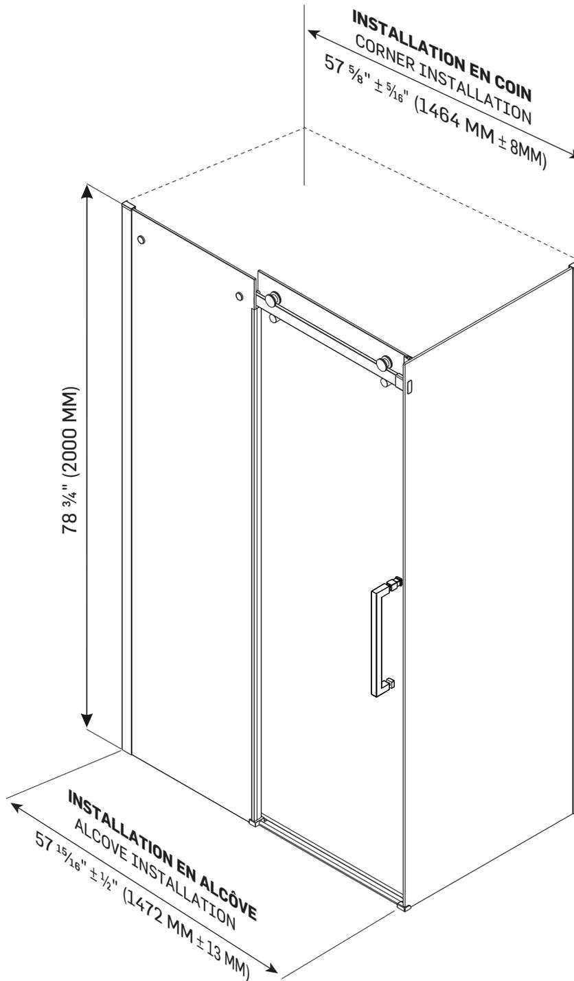
\* TOUTES CES DIMENSIONS SONT À TITRE INDICATIF. AFIN D'ASSURER UNE INSTALLATION PARFAITE, LES DIMENSIONS DE LA STRUCTURE DOIVENT ÊTRE VÉRIFIÉES À PARTIR DE L'UNITÉ AVANT L'INSTALLATION.
