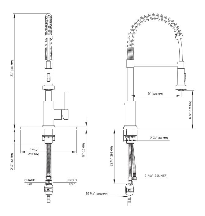
TOUTES CES DIMENSIONS SONT APPROXIMATIVES. AFIN D'ASSURER UNE INSTALLATION PARFAITE, LES DIMENSIONS DE LA STRUCTURE DOIVENT ÊTRE VÉRIFIÉES À PARTIR DE L'UNITÉ AVANT L'INSTALLATION.
