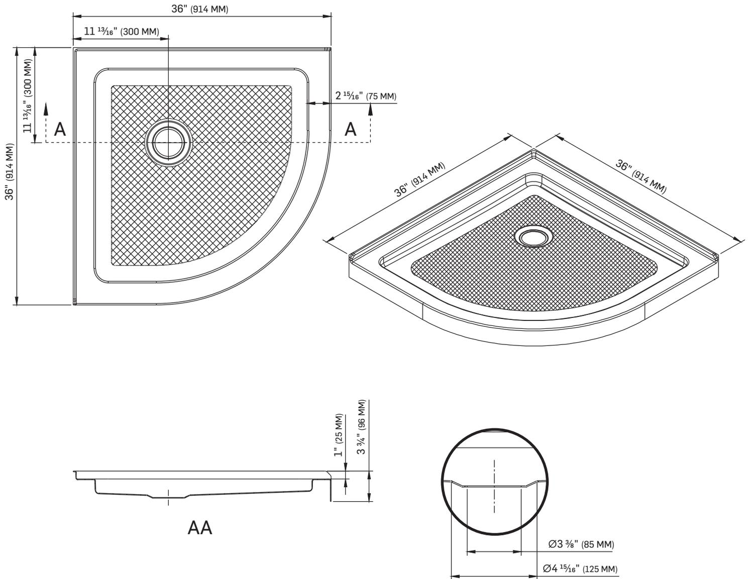
TOUTES CES DIMENSIONS SONT À TITRE INDICATIF. AFIN D'ASSURER UNE INSTALLATION PARFAITE, LES DIMENSIONS DE LA STRUCTURE DOIVENT ÊTRE VÉRIFIÉES À PARTIR DE L'UNITÉ AVANT L'INSTALLATION.
