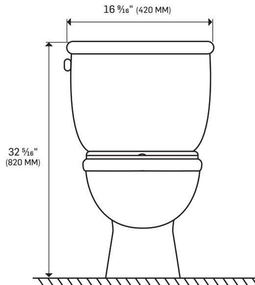
TOUTES CES DIMENSIONS SONT À TITRE INDICATIF. AFIN D'ASSURER UNE INSTALLATION PARFAITE, LES DIMENSIONS DE LA STRUCTURE DOIVENT ÊTRE VÉRIFIÉES À PARTIR DE L'UNITÉ AVANT L'INSTALLATION.
