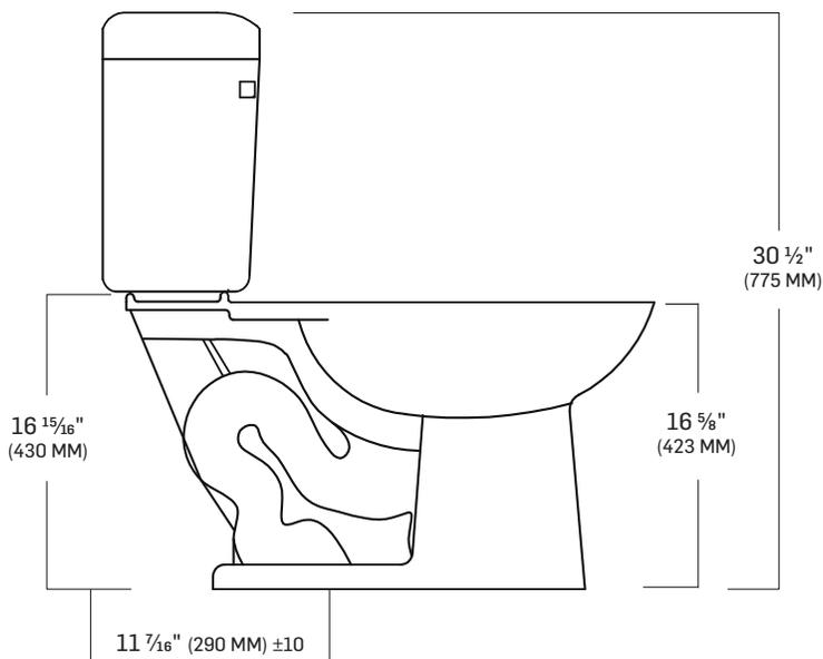
TOUTES CES DIMENSIONS SONT À TITRE INDICATIF. AFIN D'ASSURER UNE INSTALLATION PARFAITE, LES DIMENSIONS DE LA STRUCTURE DOIVENT ÊTRE VÉRIFIÉES À PARTIR DE L'UNITÉ AVANT L'INSTALLATION.
