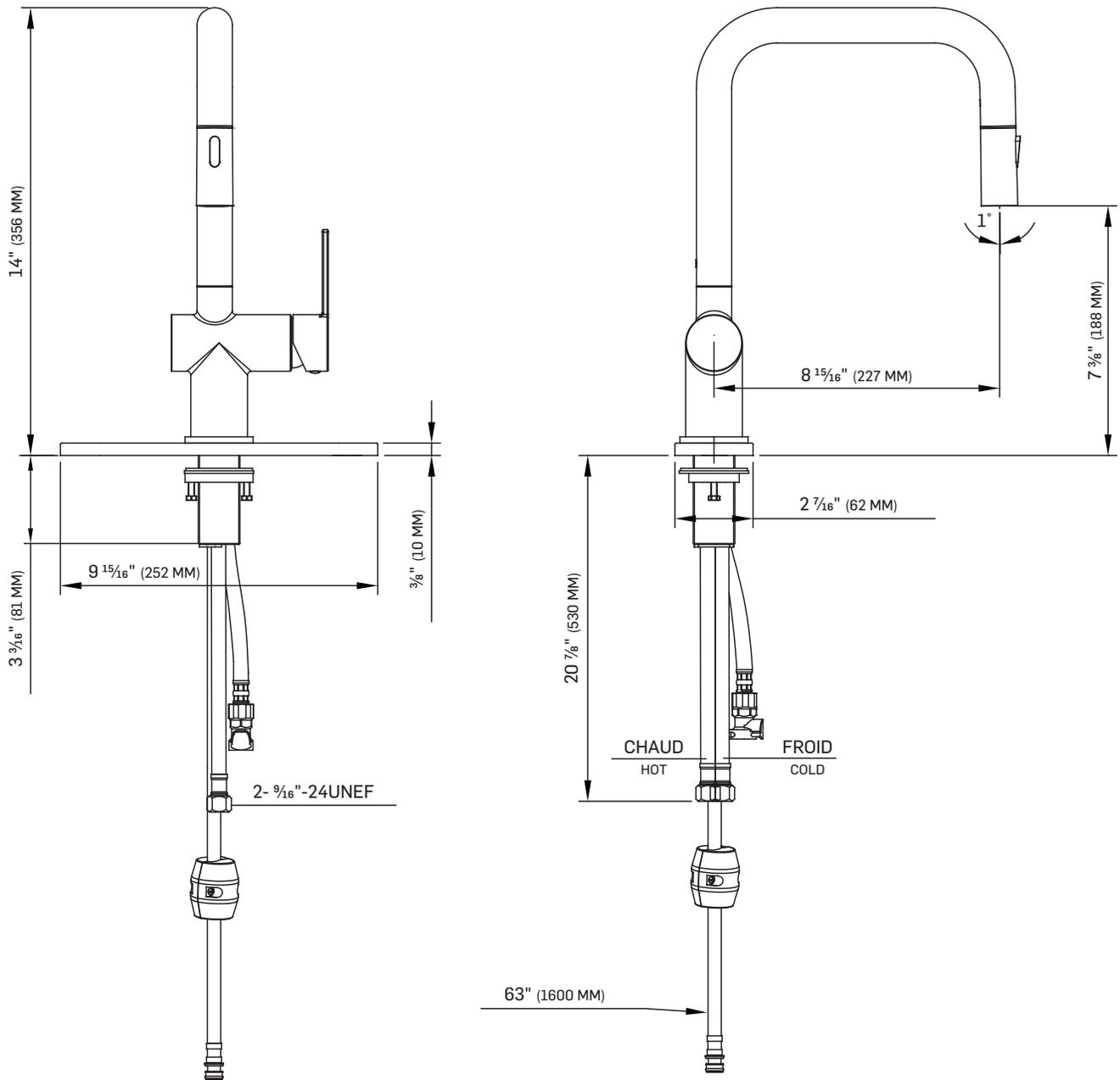
TOUTES CES DIMENSIONS SONT À TITRE INDICATIF. AFIN D'ASSURER UNE INSTALLATION PARFAITE, LES DIMENSIONS DE LA STRUCTURE DOIVENT ÊTRE VÉRIFIÉES À PARTIR DE L'UNITÉ AVANT L'INSTALLATION.
