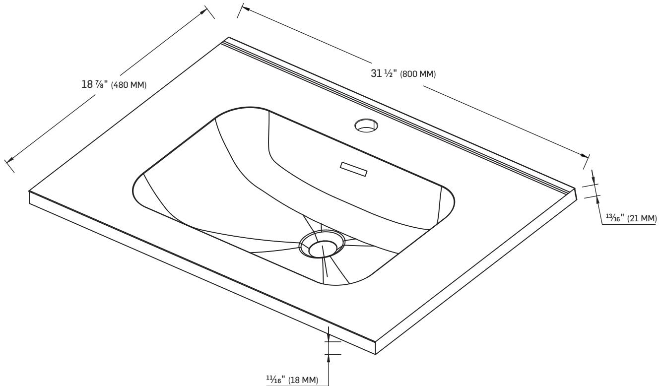
\* TOUTES CES DIMENSIONS SONT À TITRE INDICATIF. AFIN D'ASSURER UNE INSTALLATION PARFAITE, LES DIMENSIONS DE LA STRUCTURE DOIVENT ÊTRE VÉRIFIÉES À PARTIR DE L'UNITÉ AVANT L'INSTALLATION.
