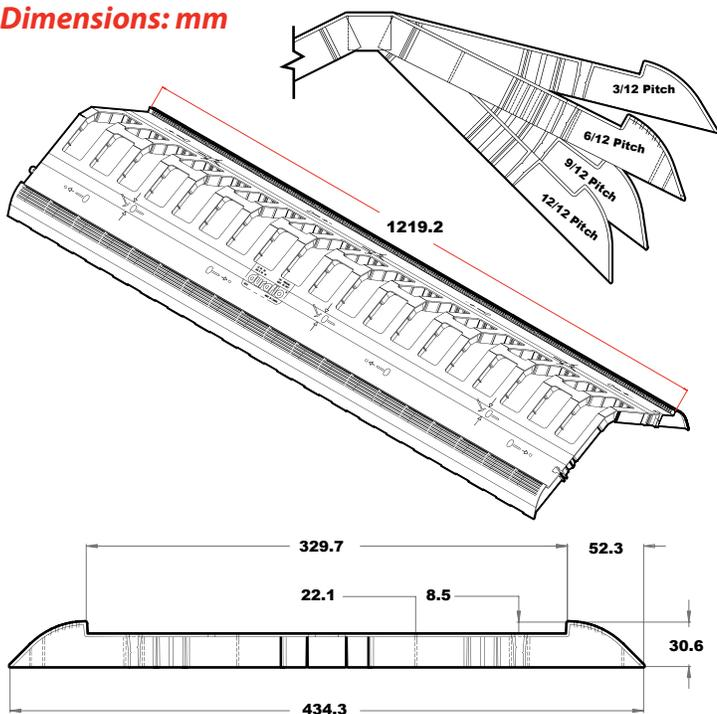
Shingles install into recessed top, allowing cleaner installation appearance while maximizing airflow over ridge.
