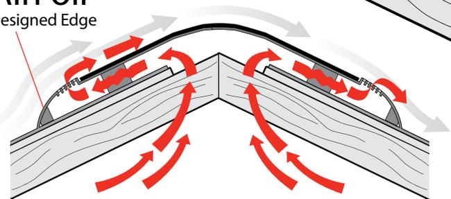
PRORidge Airfoil designed edge allows smooth airflow over the ridge line maximizing effective ventilation from the attic space while deflecting blowing debris.
