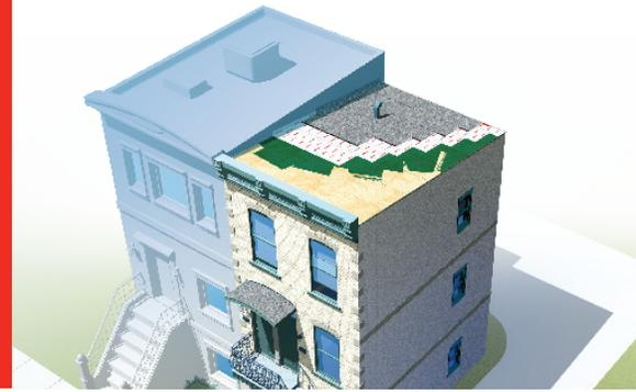
Self-adhesive granules covered finishing membrane. It is used as a finishing membrane in one-ply and two-ply waterproofing systems for low slope roofs.
