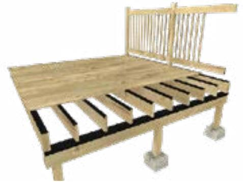
RESISTO JOIST GUARD provides waterproof protection for joists that prevents rotting of structural timber under exterior floors, such as decks and balconies. It is a self-adhesive membrane composed of elastomeric bitumen. The surface is made of polyethylene; the underside is covered with a silicone release film. 10 cm (4 in) rolls are ideal for two-inch-wide joists.
