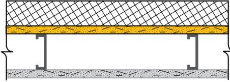
Partition Thickness: 6" – 7" (152 – 178 mm) Varies based on insulation thickness
