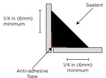
When it is not possible to use a conventional backer rod (ADSEAL BACKER ROD), it is recommended to use an anti adhesive tape.
