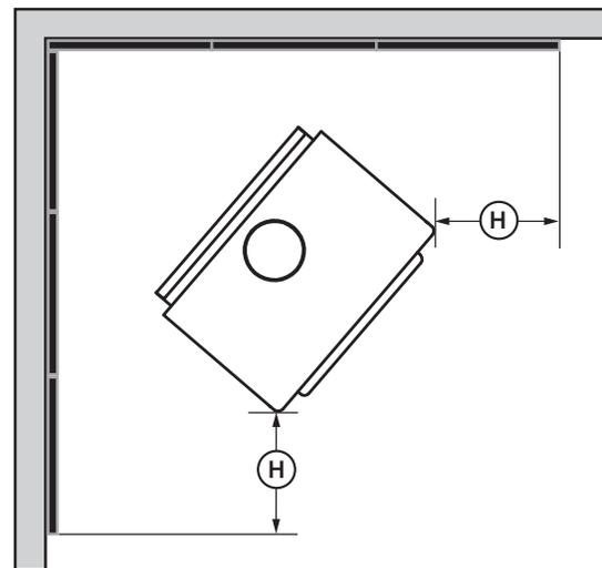
Figure 14: Heat shield clearances
