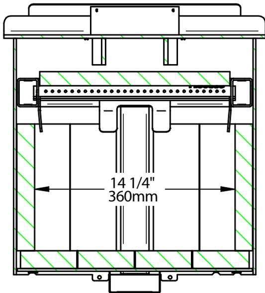
Figure 5: Front View - Combustion Chamber
