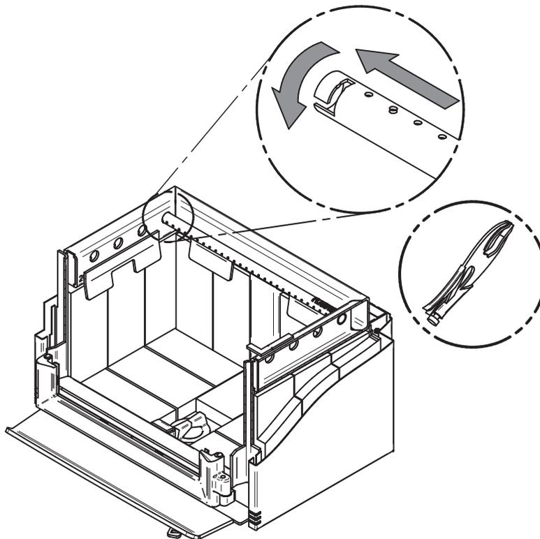
3. Put the baffle in place.
