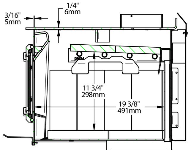
Figure 6: Side View - Combustion Chamber
