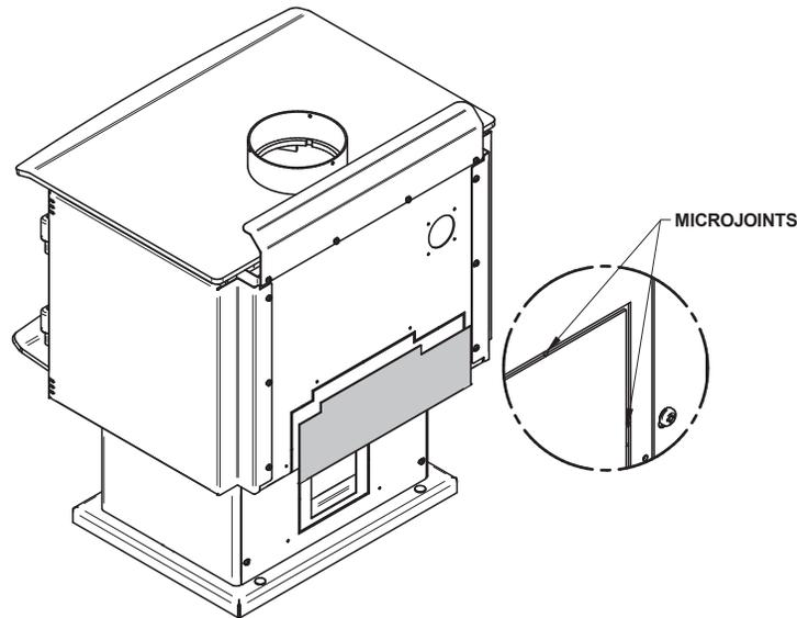
2. Screw the blower **(D)** in place using the screws **(C)** included in the installation manual. Screw the thermodisc **(A)** with the screws **(B)** supplied with the thermodisc on the back of the stove. **Ensure that the blower's power cord is not in contact with any surface of the stove to prevent electrical shock or fire damage. Do not run the power cord beneath the stove.**
