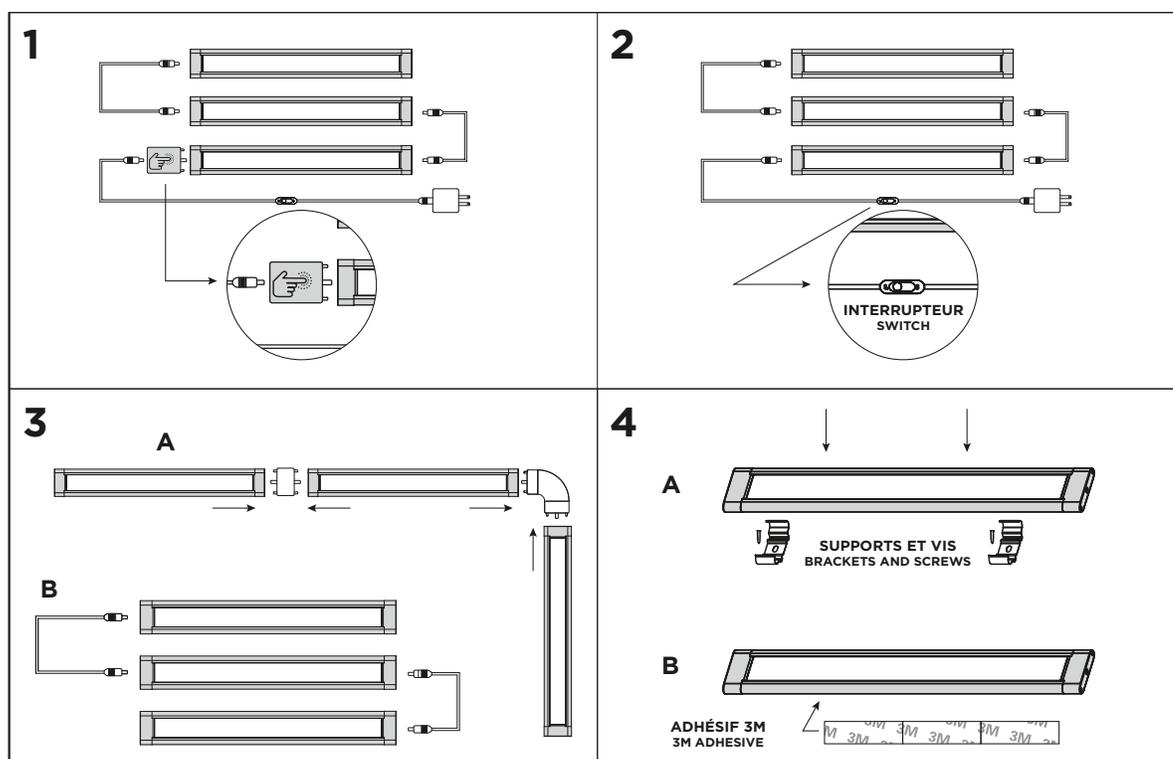
1. The dimmer switch can only be connected at this end. When connecting the light bars with the dimmer switch, you get three light intensities (6%, 50% and 100%).
