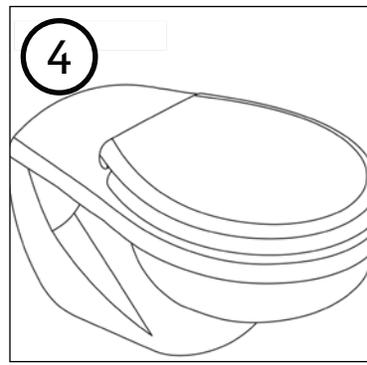
Reattach the seat: place it in a vertical position push it onto the fittings until you hear a click.
