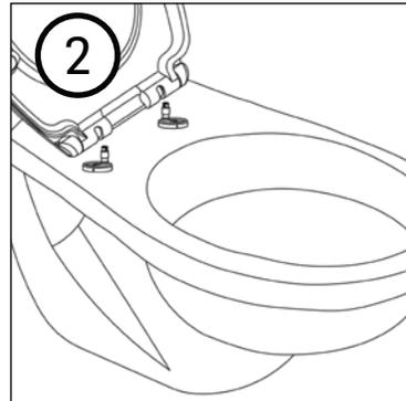
With the toilet seat in vertical position, push it onto the fittings and adjust the seat position to the toilet bowl.
