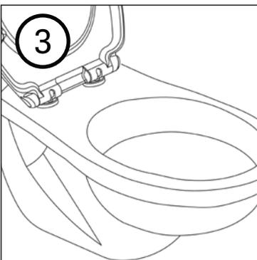
Remove the seat by lifting it vertically, tighten fittings, and cover them with caps.
