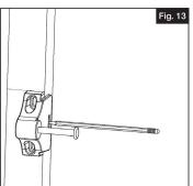
Pre-drill with 1/s" drill and then install striker with screws (Fig. 14). Check alignment with latch and adjust striker height if needed.
