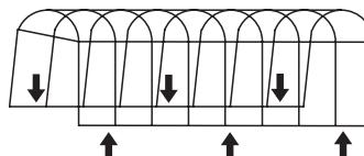
Put the anchors as show in the schema. The number of anchors depends upon the lenght of the shelter.
