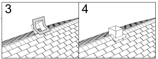
Install a bitumen sealant under the flange. all the way around, approx. 3-4" wide.
