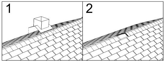
Place ridge flashing over the desired location making sure it is positioned between the rafters. Using the duct as a template, trace a line around the inside perimeter of the duct onto the shingles or deck.
