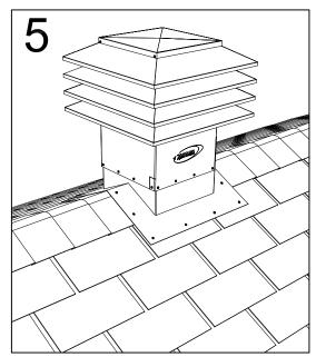
Install ventilator head onto the flashing, making sure it is level and secure to the flashing using screws provided into each of the perforations. (Model 301 shown)
