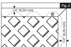
Along the sides and bottom, drill holes and put screws through molding only. Allow a 1/4" gap on all sides for expansion with cap and divider moldings (Fig. 3).
