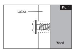
Hang the lattice with a support every 24" (Fig. 2). Attach sides and bottom loosely. (Do not tighten all the way). Do not use countersink screws.
